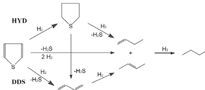
Fig (1): Reaction scheme for thiophene hydrodesulphurization
