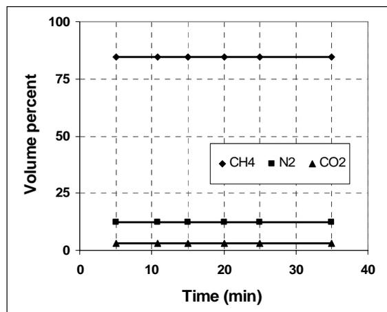
Figure 2 Gas composition versus time in batch system
