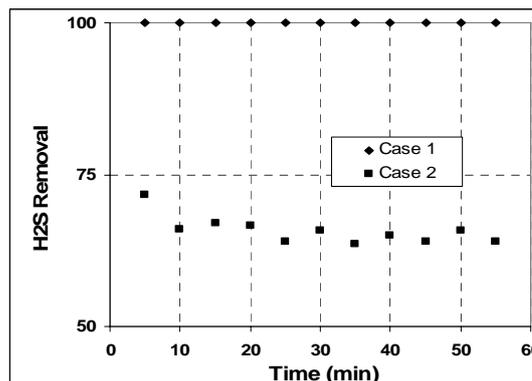
Figure 4 The pressure effect for H<sub>2</sub>S adsorption by Fe-EDTA solution
