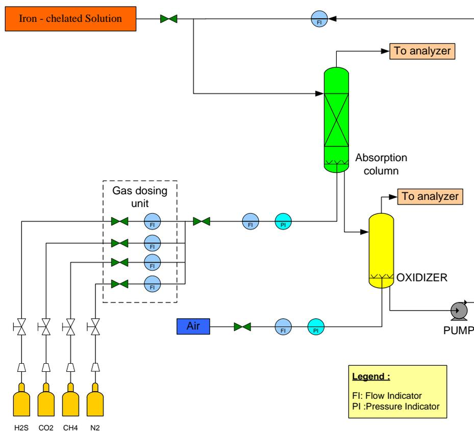
Figure 1 Schematic of laboratory set-up
