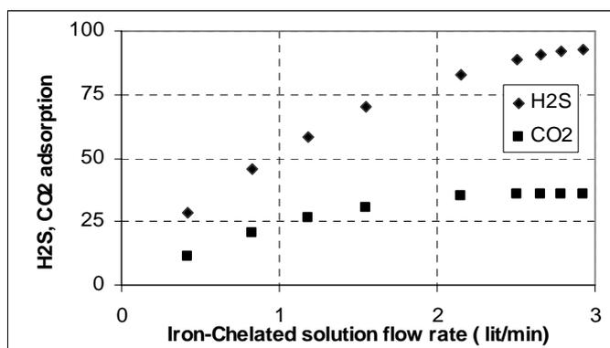
Figure 3 H<sub>2</sub>S, CO<sub>2</sub> removal versus Fe-EDTA solution flow rate
