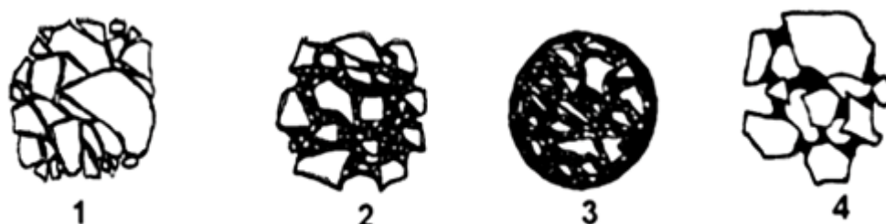
Figure 1. Main types of structures of coal-oil aggregates. The illustrations were prepared from observations through the eyepiece of MBS-9, NEOPHOT-21 microscopes.
