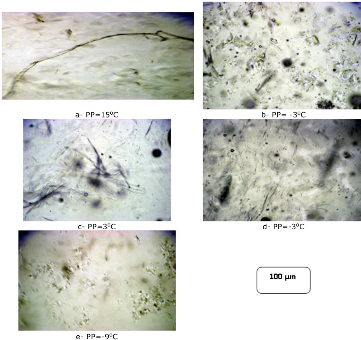
Figure 2. Photomicrographs of a: Fuel oil (FO) untreated, b: FO +200ppm (I), c: FO +200ppm (II), d: FO +200ppm (I+II) and e: FO +200ppm (I+II+III)
