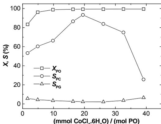
Fig. 1 Dependence of PO conversion (X) and selectivity (S) of the reaction to propylene carbonate ( $S_{PC}$ ) and to propylene glycol moieties ( $S_{PG}$ ) on the amount of the cocatalyst in the system DMF- $\text{CoCl}_2 \cdot 6 \text{H}_2\text{O}$  at  $120 \pm 2^\circ\text{C}$  and reaction time 3h
