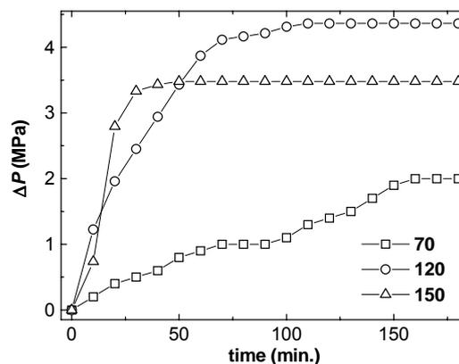
Fig. 4 Time dependence of pressure decrease (□) in the synthesis of PC (for reaction conditions see Table 3)
