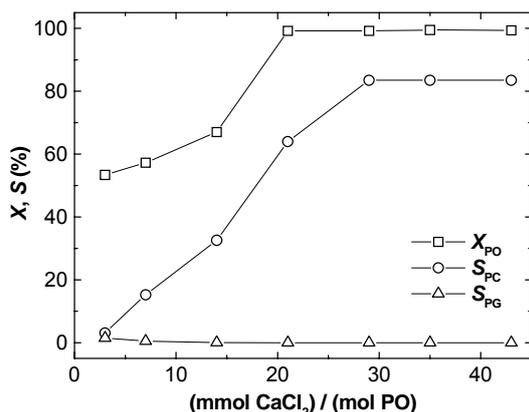
Fig. 3 Dependence of PO conversion (X) and selectivity (S) of the reaction to propylene carbonate (S<sub>PC</sub>) and to propylene glycol moieties (S<sub>PG</sub>) on the amount of CaCl<sub>2</sub> in catalytic DMF-CaCl<sub>2</sub> system (120 ± 2°C, 2.5 MPa CO<sub>2</sub> pressure and reaction time 3 h).
