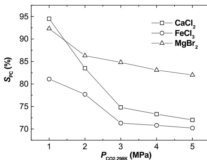
Fig. 5 Effect of initial CO<sub>2</sub> pressure (P<sub>CO<sub>2</sub>,298K</sub>) on the selectivity (S<sub>PC</sub>) to propylene carbonate .
