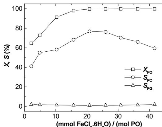
Fig. 2 Dependence of PO conversion (X) and selectivity (S) of the reaction to propylene carbonate ( $S_{PC}$ ) and to propylene glycol moieties ( $S_{PG}$ ) on the amount of  $\text{FeCl}_3 \cdot 6 \text{H}_2\text{O}$  in the catalytic system with DMF ( $120 \pm 2^\circ\text{C}$ , 2.5 MPa  $\text{CO}_2$  pressure and reaction time 3 h)
