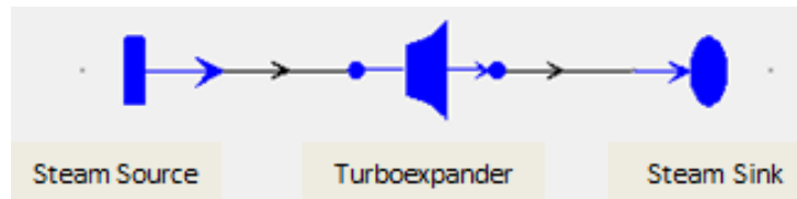
Figure3. Alternative schematic for reducing pressure of steam stream for every line
