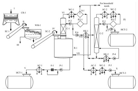
Figure 1. A schematic diagram of obtaining components of technological and boiler fuel: I - polymeric raw materials; II - crushed raw materials; III - wastewater; IV - washed and dried raw materials; V - fraction (> 360°C); VI - not stable fraction (b.p.- 360°C); VII - hydrocarbon gases; VIII - stable fraction (b.p. - 360°C); IX - fraction (b.p.-200°C); X - fraction (200-360°C)
