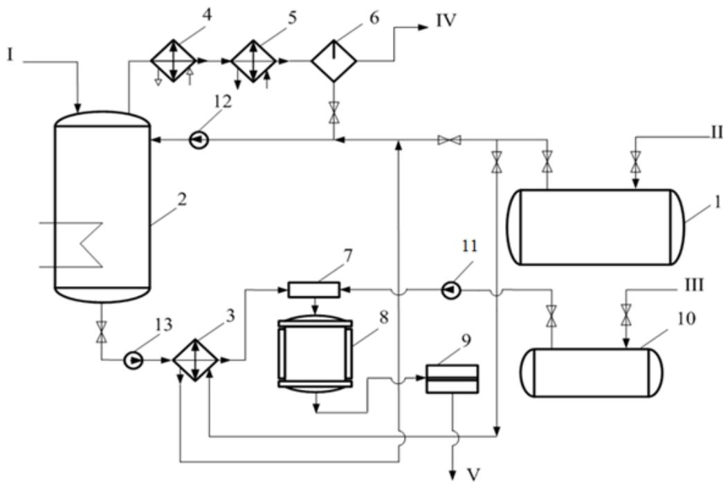
Figure 2. The principle scheme of obtaining greases from secondary raw materials: 1, 10 – containers; 2 – reactor; 3, 4, 5 – heat exchangers; 6 – separator; 7 – mixer; 8 – cooler; 9 – homogenizer; 11, 12, 13 – pumps; I – crushed polymer; II – solvent (dispersion medium); III – anti-corrosion additive; IV – gases of destruction; V – grease
