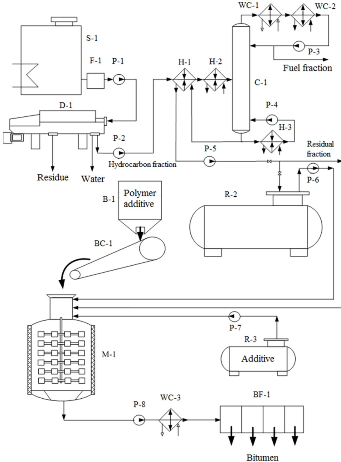
Fig. 2. Technological scheme of modified bitumen production
