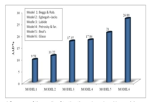
Figure 4 Summary of the results of testing the various viscosities models
