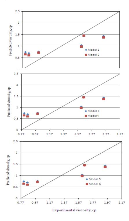
Figure 2 Statistical accuracy of the investigated dead oil viscosity correlations
