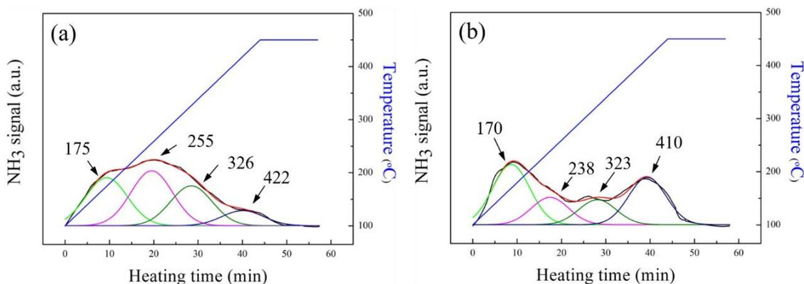
Fig. 5. NH<sub>3</sub>-TPD profiles of (a) Cu-SSZ-13-25, (b) Cu-SSZ-13-25 after SO<sub>2</sub> and water vapor poisoning experiment.
