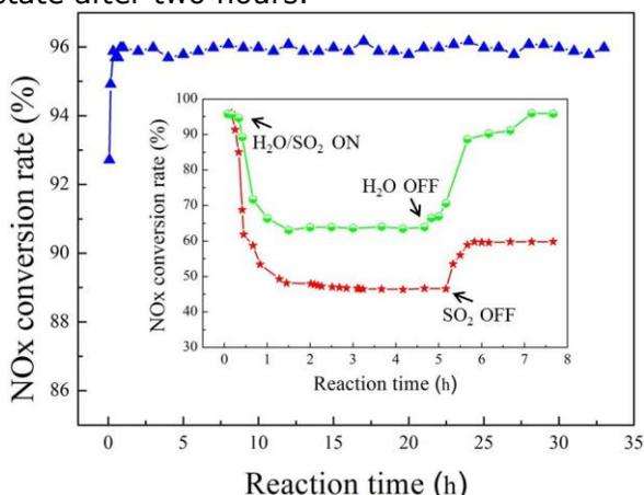
Fig. 4. The life test and the effect of SO<sub>2</sub> and water vapor on the SCR activities of the Cu-SSZ-13-25 catalyst. All Reaction was conducted at 300 °C
