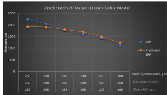
Fig. 7. Measured SPP vs. predicted SPP using Hassan and Kabir model.
