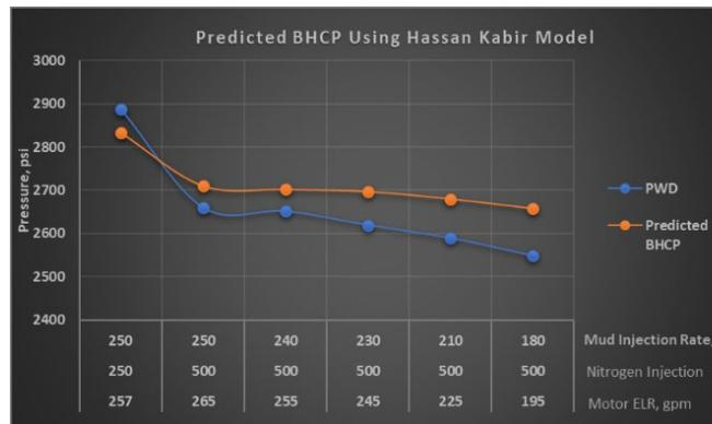
Fig. 5. Measured wellbore pressure vs. predicted BHCP using Hassan & Kabir model.
