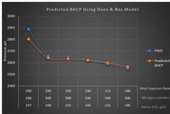
Fig. 4. Measured wellbore pressure vs. predicted BHCP using Duns and Ros model.
