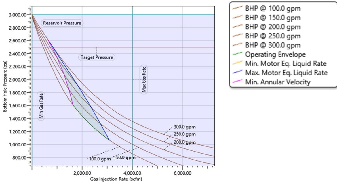
Fig. 8. UBD operating envelope of well 112-78H.
