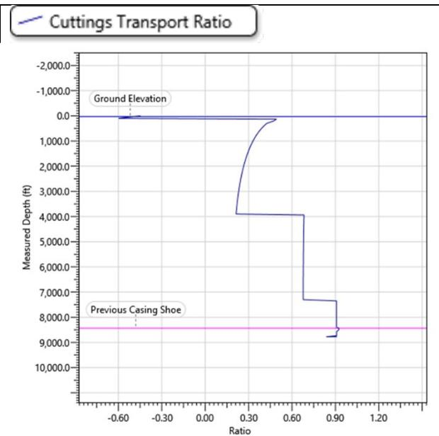
Fig. 11. Cutting transport ratio at the recommended operating condition and 100 psi choke back pressure.
