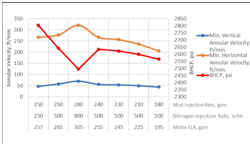
Fig. 9. Comparison of different operating conditions of well 112-78H.
