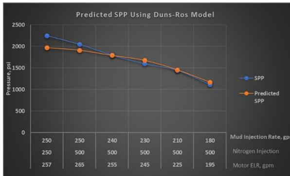
Fig. 6. Measured SPP vs. predicted SPP using Duns and Ros model.
