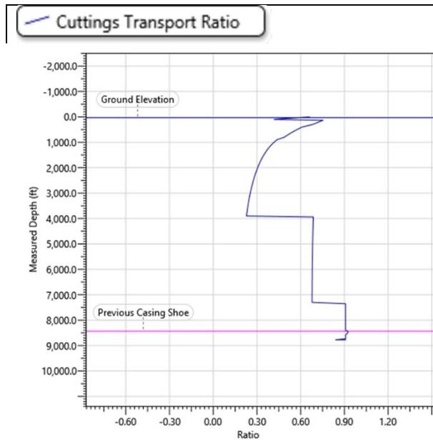
Fig. 10. Cutting transport ratio at the recommended operating condition and zero choke back pressure.
