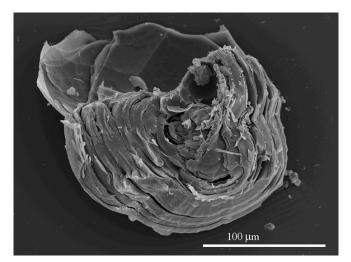
Fig. 3. Destroyed cluster of the carbon deposit from the coke oven chamber
