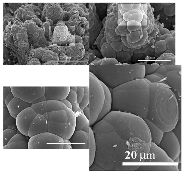
Fig. 1 (a,b,c). The fractal structure of the carbon Fig. 2. Multi-layer structure of the cluster from the coke deposits from the coke oven at different magnifications
