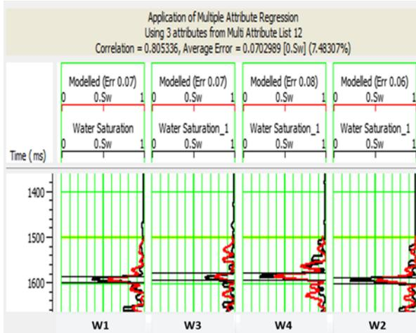
Figure 4. Modelled versus measured water saturation at the location of four wells (W1, W2, W3, W4) using multi attributes with correlation of 0.8
