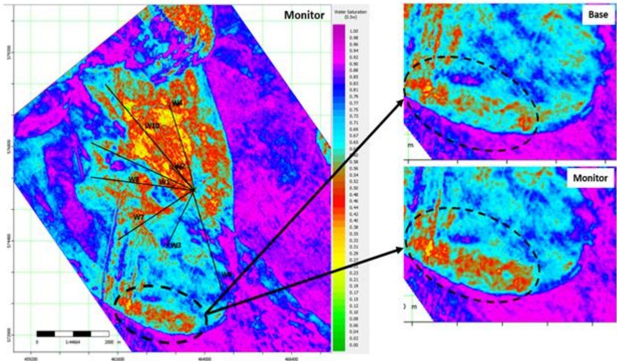
Figure 7. Water saturation map of monitor survey indicates detecting remain oil in regions that oil swept as a result of water injection. Lower values of water saturation compare to base survey
