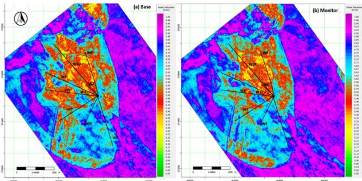
Figure 5 Predicted water saturation for (a) base and (b) monitor survey using neural network at the reservoir interval indicates replacement of oil by water at location of injection wells and distribution of water in reservoir
