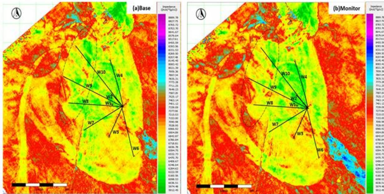
Figure 3. Acoustic impedance map of (a) base and (b) monitor survey indicates Hardening effect in reservoir after water replacing oil and Increase in acoustic Impedance in monitor survey
