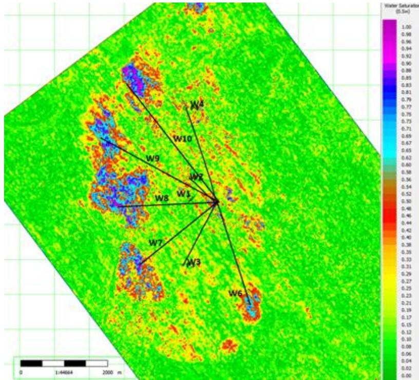
Figure 6. Difference map (monitor-base) shows higher values of water accumulation at the location of injection wells
