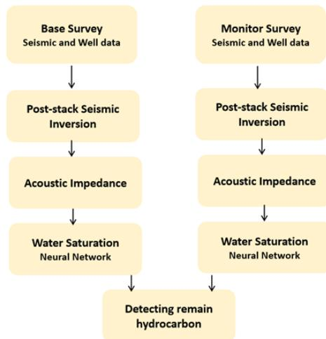
Figure 2. Overall workflow of qualitative 4D seismic study for water saturation prediction
