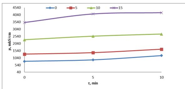
Fig. 6. Dependence of conductivity of the solutions of polyvinyl alcohol on the content of humic acid obtained from sample No. 2
