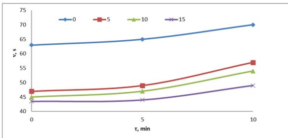
Fig. 4 Dependence of the conditional viscosity of the solutions of polyvinyl alcohol on the content of humic acid obtained from sample No. 3
