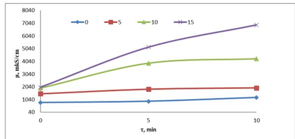
Fig. 5. Dependence of conductivity of the solutions of polyvinyl alcohol on the content of humic acid obtained from sample No. 1
