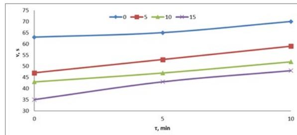
Fig. 3 Dependence of the conditional viscosity of the solutions of polyvinyl alcohol on the content of humic acid obtained from sample No. 2
