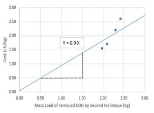
Figure 4. Graphical representation between the removing mass load of COD and the treatment cost for technique 1.
