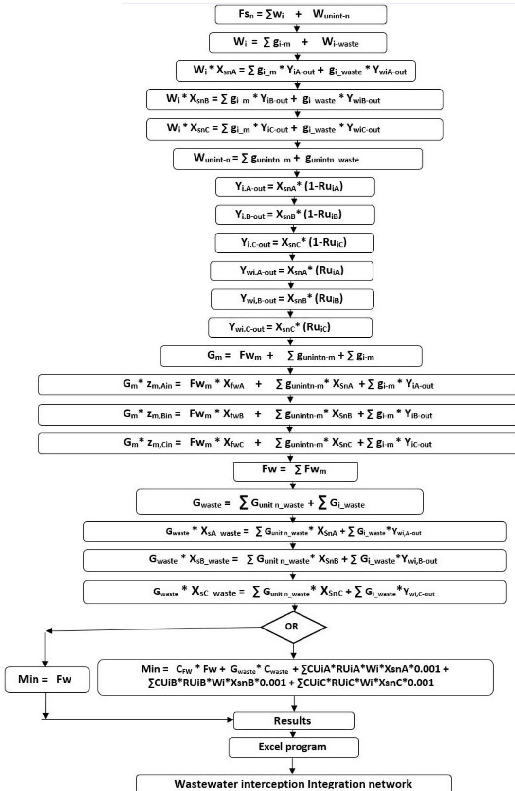
Figure 2. The procedure for designing the Wastewater interception Integration network
