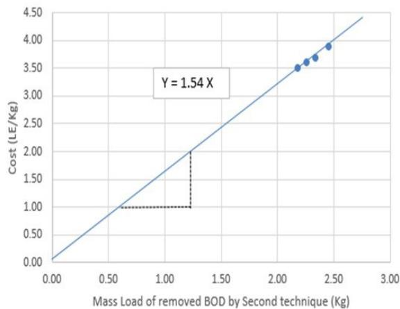
Figure 8. Graphical representation between the removing mass load of BOD and the treatment cost for technique 2
