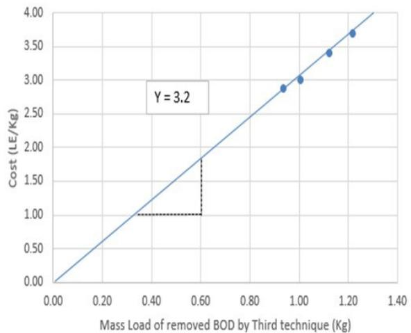
Figure 9. Graphical representation between the removing mass load of BOD and the treatment cost for technique 3
