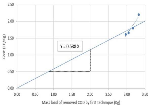
Figure 4. Graphical representation between the removing mass load of COD and the treatment cost for technique 1.
