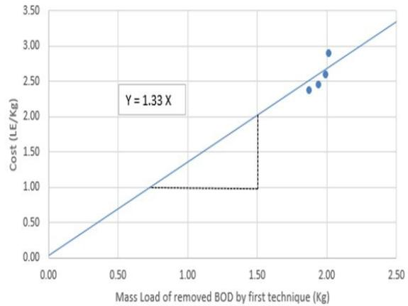
Figure 7. Graphical representation between the removing mass load of BOD and the treatment cost for technique 1
