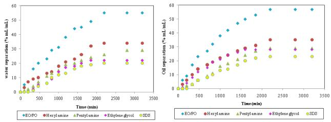
Fig. 1. The effect of different demulsifiers on crude oil emulsion stability (percentage of water separation) Fig. 2. The effect of different demulsifiers on crude oil emulsion stability (percentage of oil separation)
