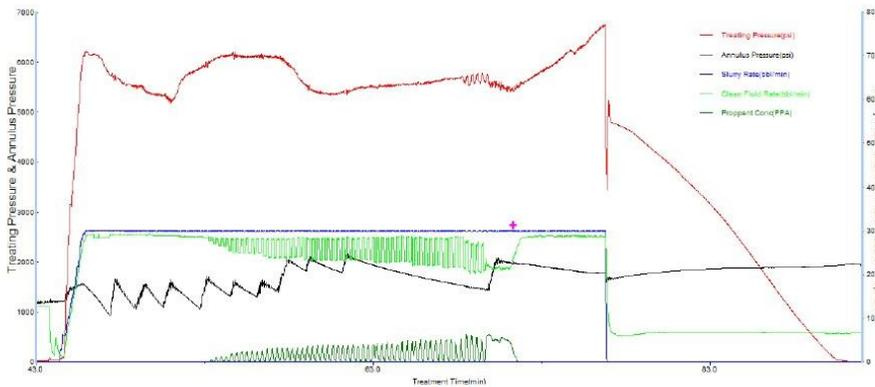
Figure 9. Pressure response of the first step of dual fracturing on P1
