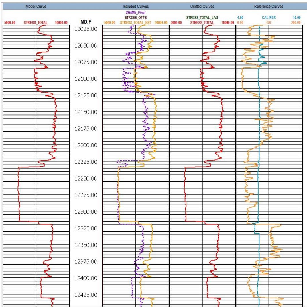
Figure 4. Stress profile for stimulation design which is created by dipole sonic log processing of offset Well P-05
