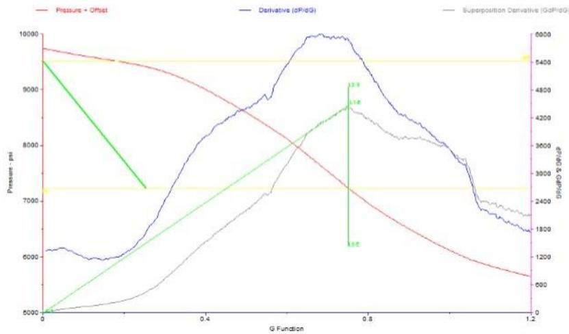
Figure 8. G-Function analysis of the first step of dual fracturing on P1
