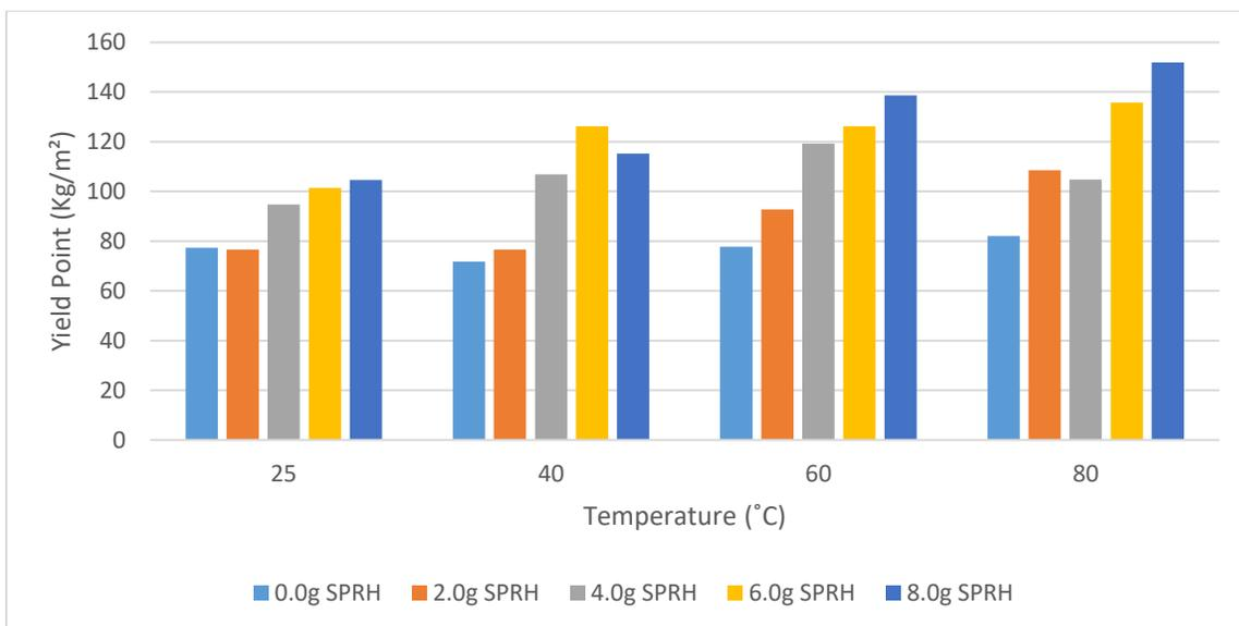
Figure 2. Yield point of SPRH starch mud compositions at different temperature
