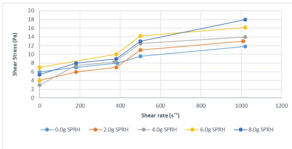
Figure 8. Rheogram illustrating the fluid behaviour at a temperature of 60°C
