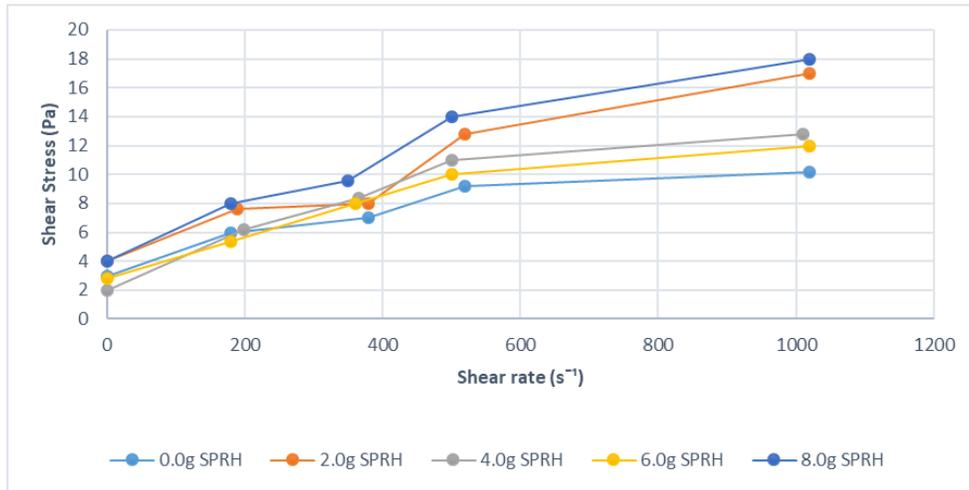
Figure 6. Rheogram illustrating the fluid behaviour at a temperature of 25°C
