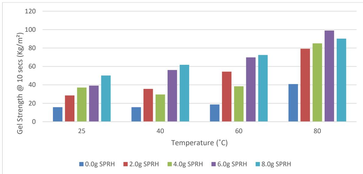
Figure 3. Ten seconds gel strength of SPRH starch mud compositions vs temperature
