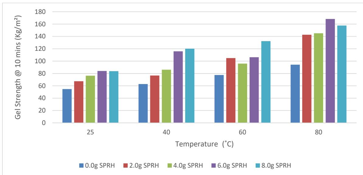
Figure 4. Ten minutes gel strength of SPRH starch mud compositions vs temperature
