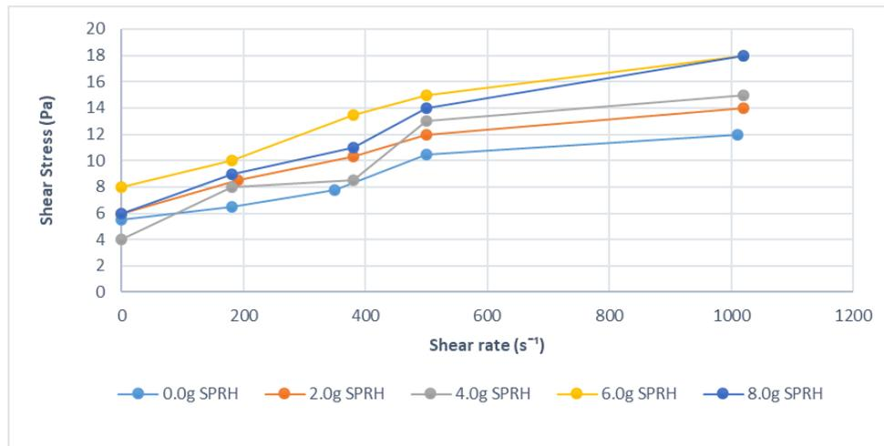
Figure 9. Rheogram illustrating the fluid behaviour at a temperature of 80°C
