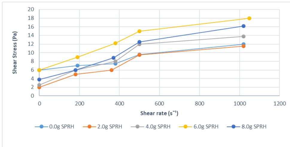
Figure 7. Rheogram illustrating the fluid behaviour at a temperature of 40°C
