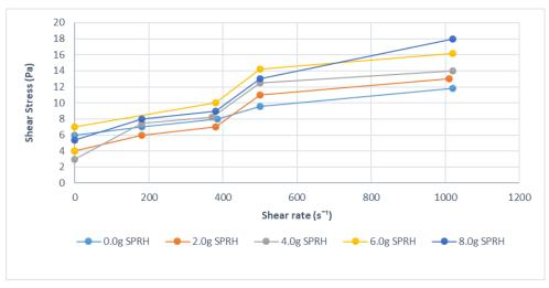
Figure 8. Rheogram illustrating the fluid behaviour at a temperature of  $60\degree C$
