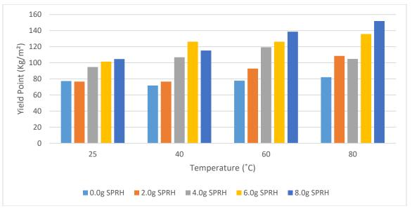
Figure 2. Yield point of SPRH starch mud compositions at different temperature
