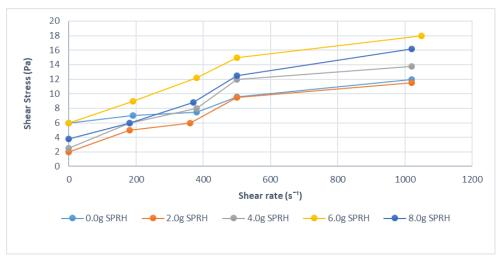
Figure 6. Rheogram illustrating the fluid behaviour at a temperature of  $25^{\circ}C$
