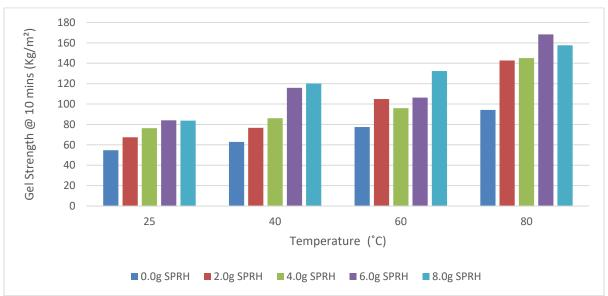
Figure 3. Ten seconds gel strength of SPRH starch mud compositions vs temperatur
