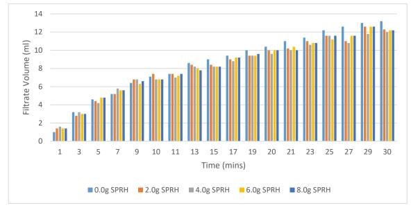
Figure 5. Filtration Loss of the Samples of Mud vs Time
