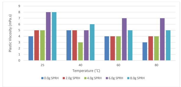
Figure 1. Plastic viscosity of the SPRH composition at different temperature
