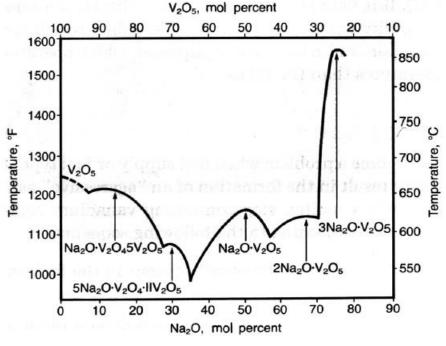
Fig.3- Vanadium oxides and its melting points
