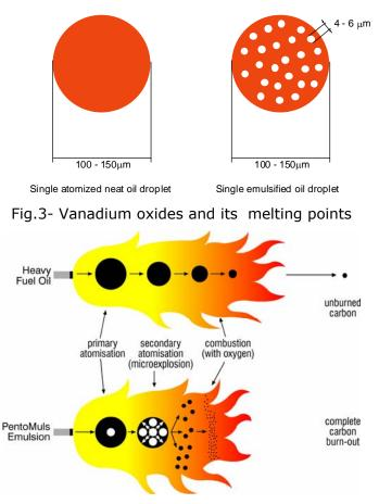
Fig.2: Combustion with and without water-in-oil emulsion
