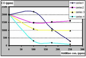
Fig 8. Chemical additives effect on emission of gas CO Series 1. Cu, Series 2. Mn, Series 3. Mn+Cr Series 4. Cu+ Mn+Cr
