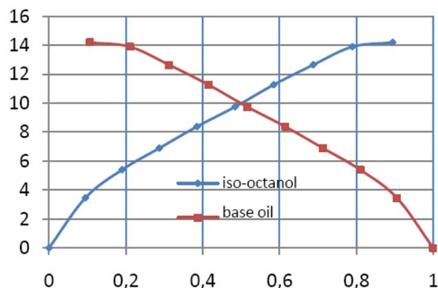
Fig 3 Excess volume of gas oil spiked /iso-octanol systems.
