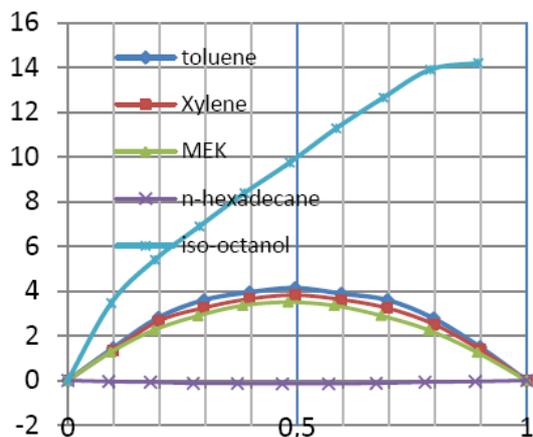
Figure 2 Excess volume of spiked gas oil.
