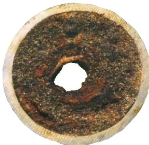
Fig.1. Wax deposited in the pipe
