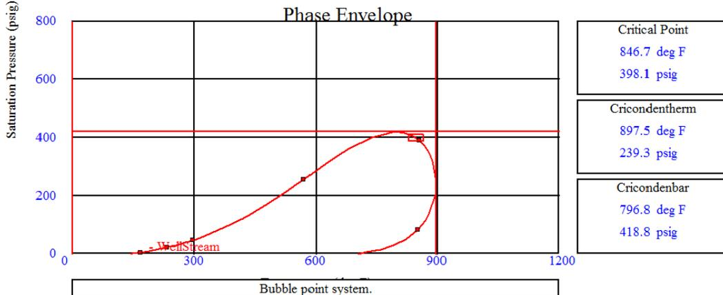
Figure 4. Phase envelope of the fluid sample
