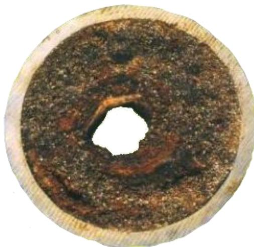
Fig.1. Wax deposited in the pipe
