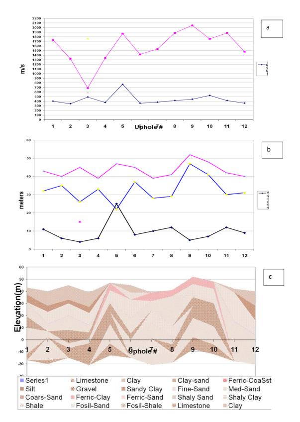
Fig. 14. Cross-sectional plots of the study area showing Up hole Shot points 1 to 12: (a) Cross section showing seismic velocity across the study area (b) Cross section showing elevation across the study area(c) Cross section showing lithology across the study are
