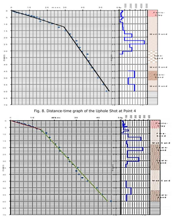
Fig. 9. Distance-time graph of Up hole Shot at Point 5
