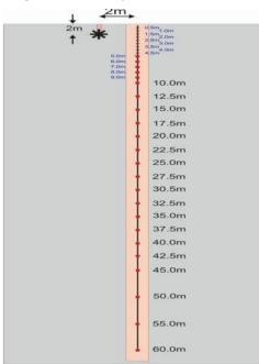
Fig. 5 Schematic diagram showing hydrophones design array
