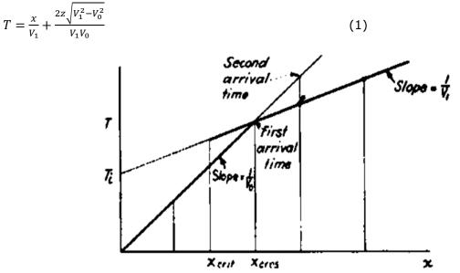
Fig 4b. Schematic diagram illustrating the path of seismic waves
