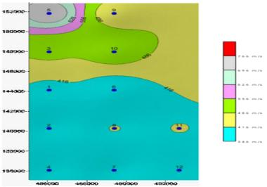
Fig. 11. Low-Velocity Layer1 (Weathering Layer) Contour Map
