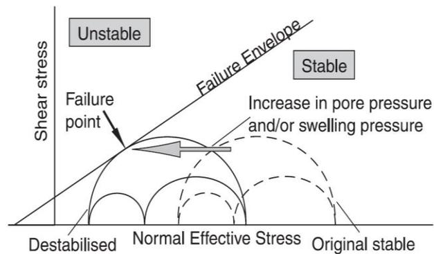
Fig.5. Mohr– Coulomb representation of shale failure: the increase in pore pressure and/or swelling pressure will reduce all effective normal stresses (note that shear stresses remain unaltered) until the stress state touches the failure envelope and the shale fails for a given orientation around the wellbore. *Reproduced after* [51]
