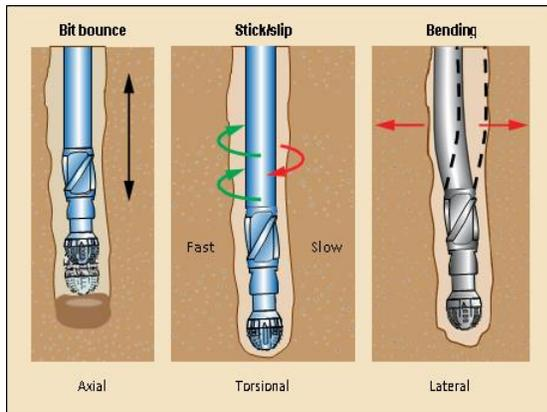
Fig.4. Types of drill string vibrations [30]
