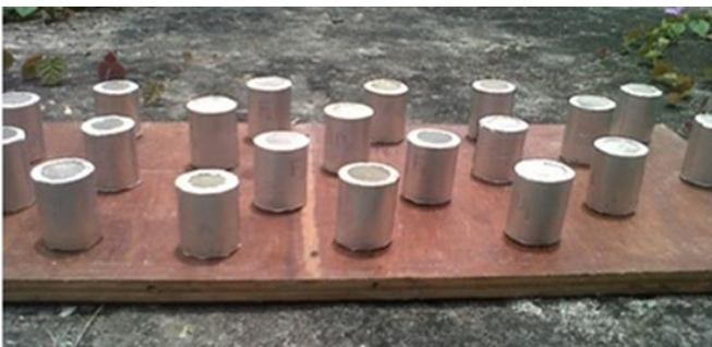
Fig. 3. Agbada sandstone reservoir core plugs used in this work
