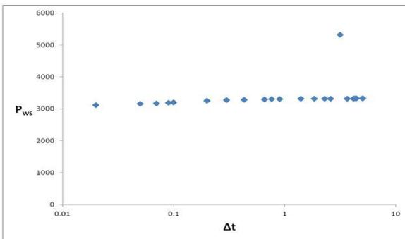
Figure 5. Plot of  $P_{ws}$  Vs  $\Delta T$  for Well 3 (Pre-Stimulation)
