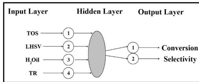
Figure 2. Simplified structure of ANN and ANFIS models developed for isomerization process
