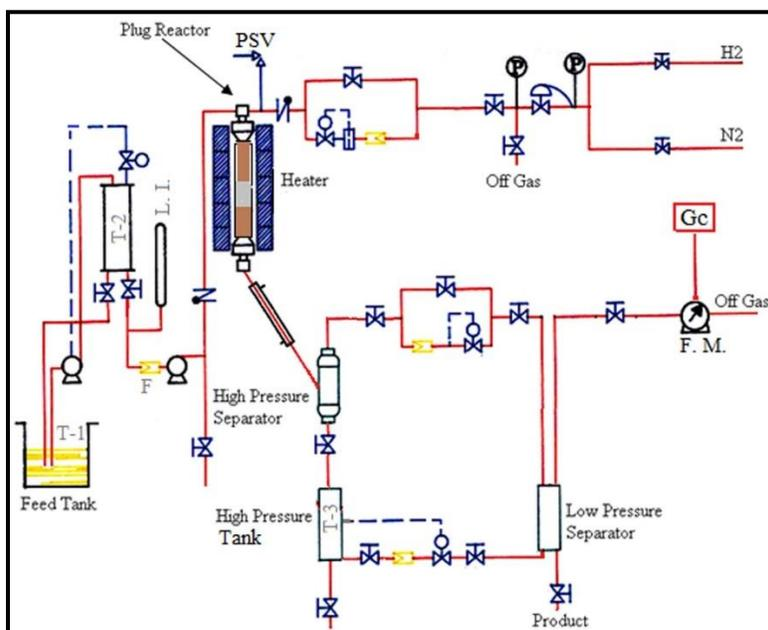
Figure 1. Flow diagram of the isomerization set up. T, storage tank; L.I., level indicator; PSV, pressure switch valve; P, pressure gauge; F, filter (mesh 40 $\mu$ m); GC, gas chromatography analyzer; F.M., flow meter [2]
