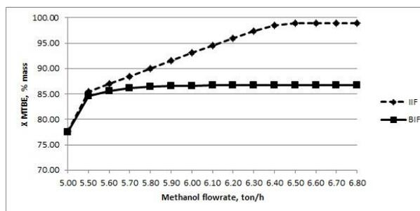
Figure 7. MTBE content as a function of methanol flowrate
