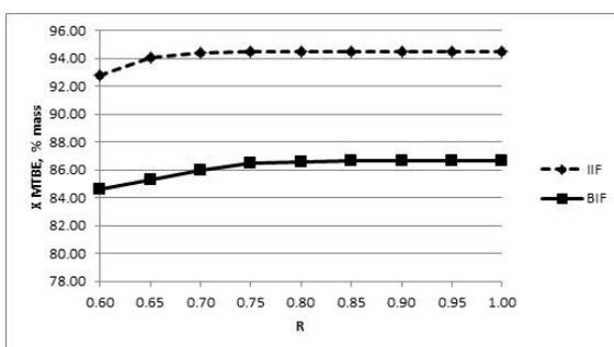
Figure 6. MTBE content as a function of reflux ratio
