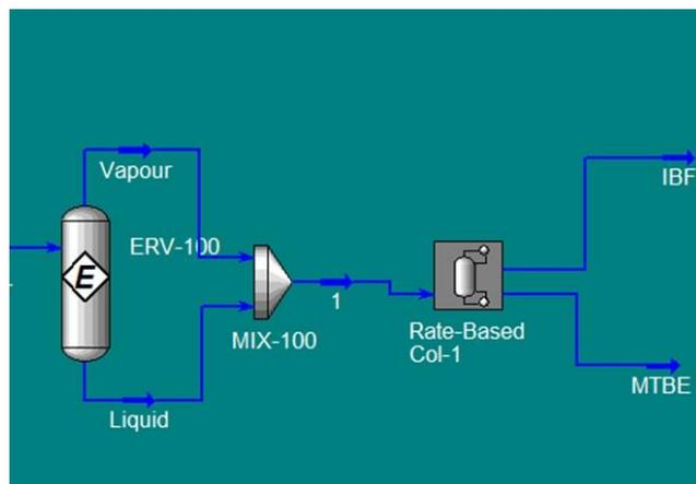
Figure 5. HYSYS® scheme of the MTBE production unit
