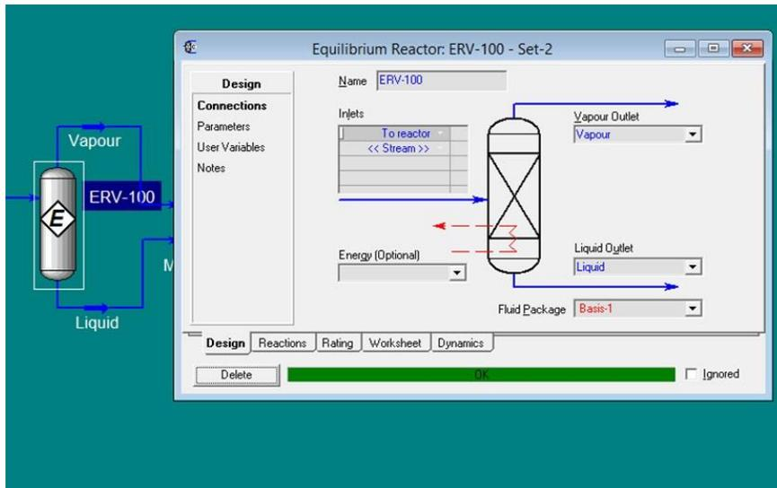
Figure 2. The MTBE synthesis reactor modeling in Aspen HYSYS®
