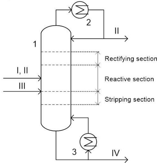
Figure 3. The reactive distillation column ( I – isobutylene; II – n-butylenes; III – methanol; IV – MTBE; 1 - reactive distillation column; 2 - total condenser; 3 – reboiler)
