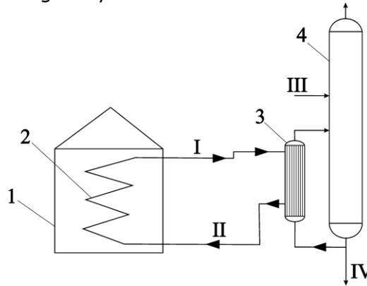
Fig. 6 Principal scheme of heating of the column cube with the heating pipe: 1 – heating furnace; 2 – evaporator of heat pipe; 3 – condenser of heat pipe; 4 – rectification column; I – coolant vapour; II – coolant condensate; III – raw material; IV – bottom stream
