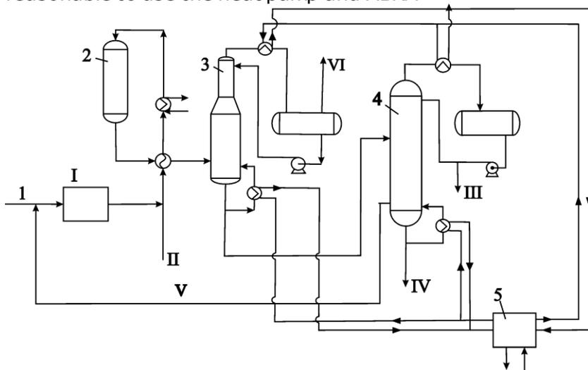
Fig. 4 – Principal scheme of isomerisation unit: 1 – dryer; 2 – reactor of isomerisation; 3 – stabilization column; 4 – deisohexanizer; 5 – ACU; I – raw material, II – hydrogen; III – isomerizate; IV – C<sub>7+</sub> fraction; V – recycled material; VI – fuel gas.
