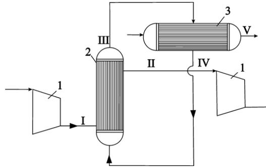
Fig. 5 – Principal scheme of gas cooling with the heat pipe: 1 – compressor; 2 – evaporator of heat pipe; 3 – condenser of heat pipe; I – hot gas; II – cold gas; III – vapour; IV – condensate; V – water
