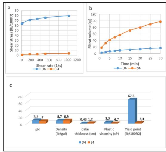
Figure 5. Comparison of rheological properties for S4 and D4 samples, a) Shear rate-shear stress relations b) Time-fluid loss relation, c) pH, density, cake thickness, plastic viscosity, yield point values
