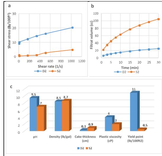
Figure 3. Comparison of rheological properties for S2 and D2 samples, a) Shear rate-shear stress relations b) Time-fluid loss relation, c) pH, density, cake thickness, plastic viscosity, yield point values
