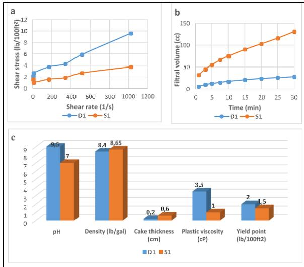
Figure 2. Comparison of rheological properties for S1 and D1 samples, a) Shear rate-shear stress relations b) Time-fluid loss relation, c) pH, density, cake thickness, plastic viscosity, yield point values
