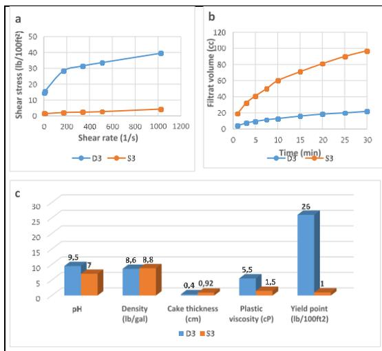
Figure 4. Comparison of rheological properties for S3 and D3 samples, a) Shear rate-shear stress relations b) Time-fluid loss relation, c) pH, density, cake thickness, plastic viscosity, yield point values
