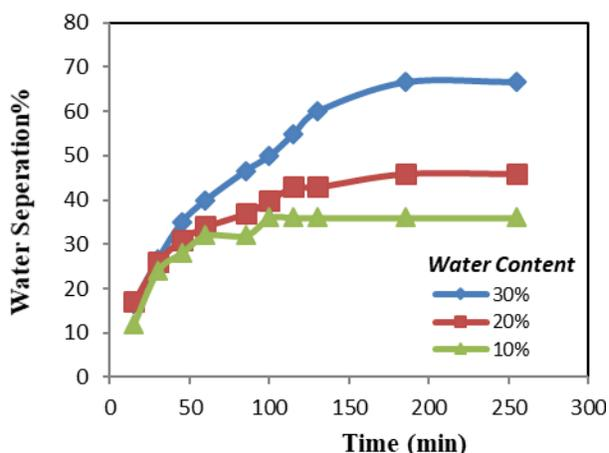
Fig. 5. Effect of water content at constant demulsifier concentration 8%, temperature 70°C and salt content 3%
