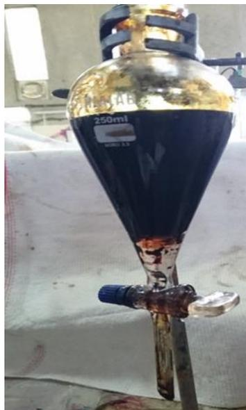
Fig. 2. Separation funnel for separate water and crude oil
