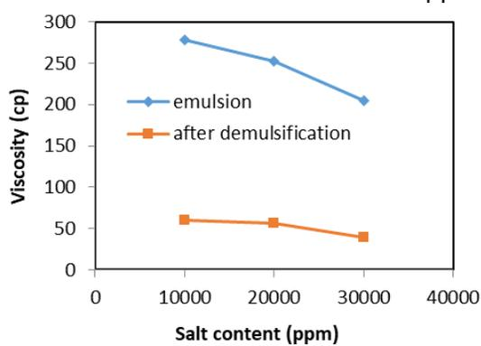
Fig. 10 Effect of salt content on viscosity at water content 30%, demulsifier concentration 8% and temperature  $70^\circ\text{C}$
