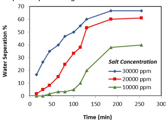
Fig. 6. Effect of salt content at constant demulsifier concentration 8%, temperature 70°C and water content 30%
