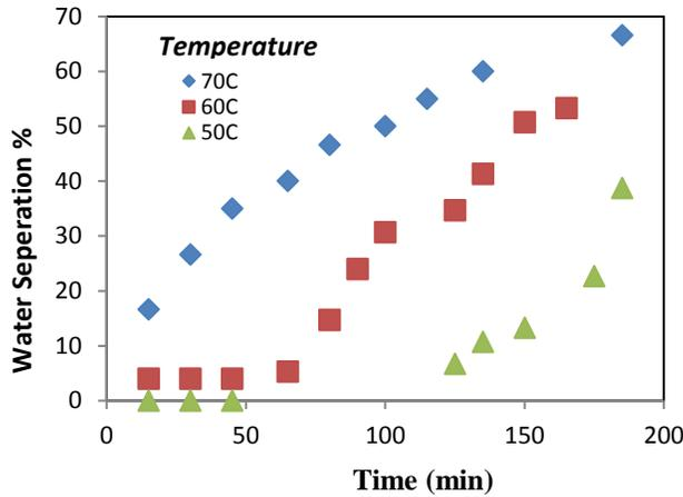
Fig. 7. Effect of temperature at constant water content 30%, salt content 3% and demulsifier concentration 8%
