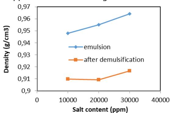
Fig. 11. Effect of salt content on density at water content 30%, demulsifier concentration 8% and temperature  $70^\circ\text{C}$
