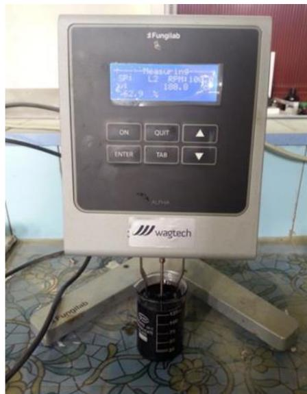
Fig. 3. Viscometer Fungilab
