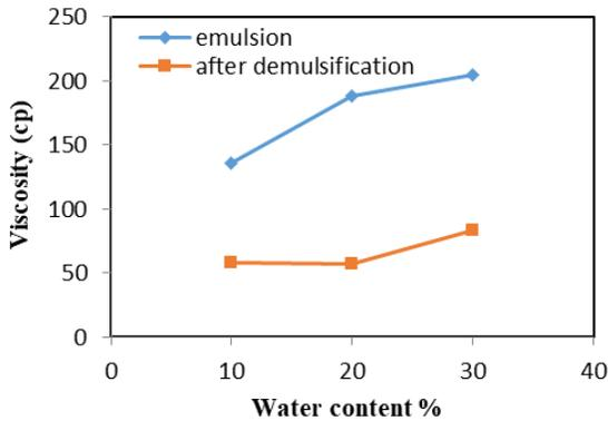
Fig. 8. Effect of water content on viscosity at salt concentration 3%, demulsifier concentration 8% and temperature 70°C
