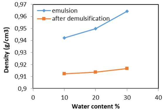
Fig. 9. Effect of water content on density at salt concentration 3%, demulsifier concentration 8% and temperature 70°C
