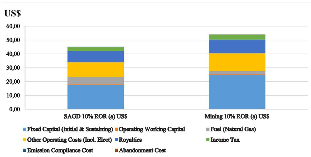
Figure 3. Breakdown of Bitumen/SCO Supply Cost (Source: CERI)
