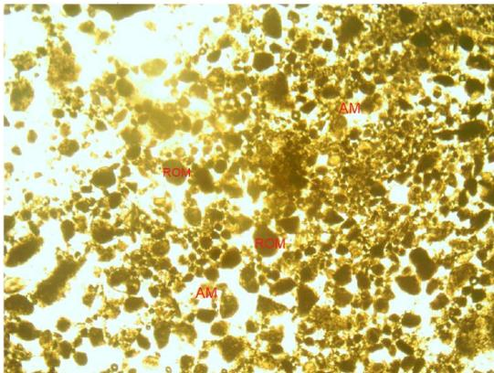
Figure 7. Photomicrograph of sample 4 (42m) (magnification: x40), ROM –recycled organic matter, AM-amorphous matter
