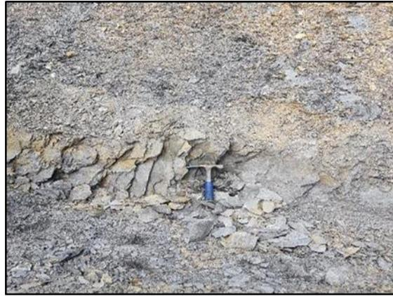
Fig. 13. Highly fractured shale with quartz and phyllite inclusions
