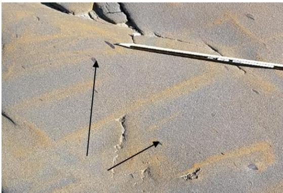
Figure 10. Fine sandstone with coal lenses from TA-3 Outcrop
