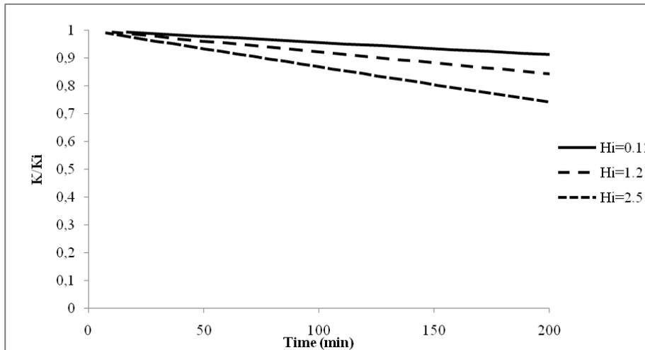
Figure 9. Effect of heterogeneity on permeability reduction.
