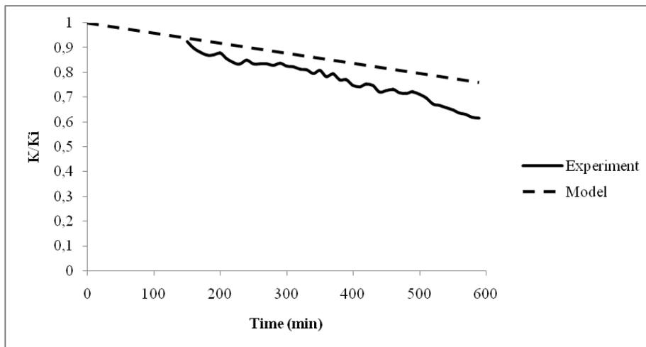
Figure 7. Permeability reduction due to asphaltene precipitation.
