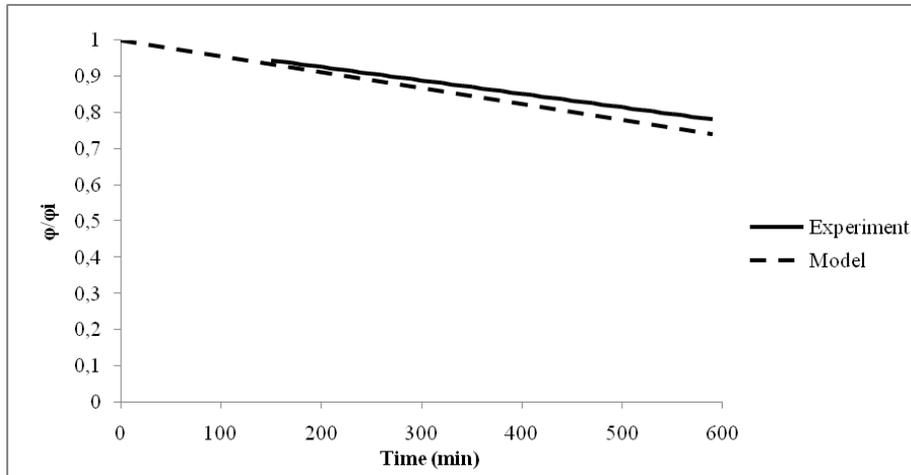
Figure 8. Porosity reduction due to asphaltene precipitation.
