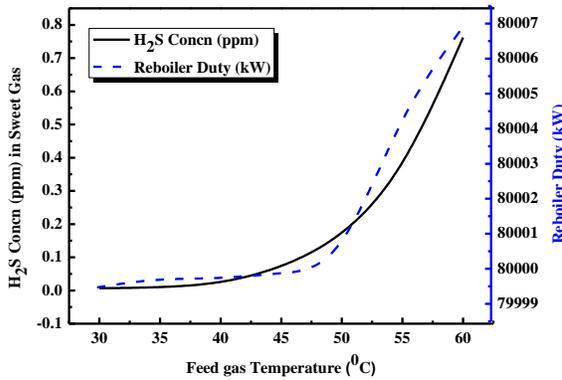
Figure 3. Effect of feed gas temperature on H<sub>2</sub>S concentration in sweet gas
