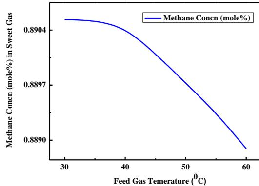
Figure 4. Effect of feed Gas temperature on methane concentration in sweet gas
