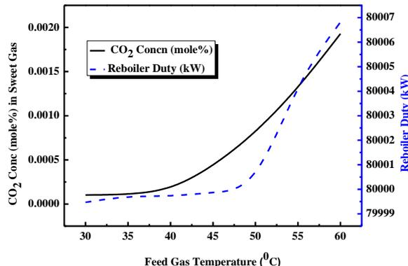
Figure 2. Effect of feed gas temperature on CO<sub>2</sub> concentration in sweet gas
