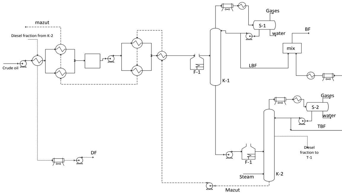
Fig. 1. Structure of crude oil distillation unit without heat integration
