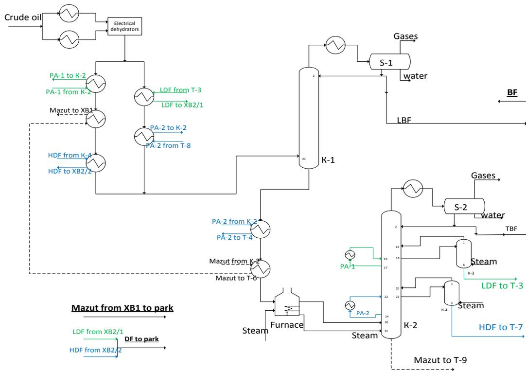
Fig. 2. Basic distillation unit with heat integration
