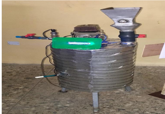
Figure 4. Developed small-scale biogas plant
