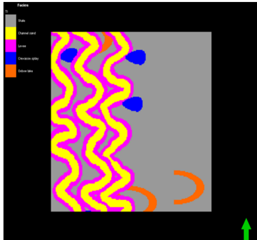
Figure 7. TI 3 – training image (map view) showing floodplain (grey), channel (yellow), levee (pink), crevasse splay (blue) and oxbow lake (orange)
