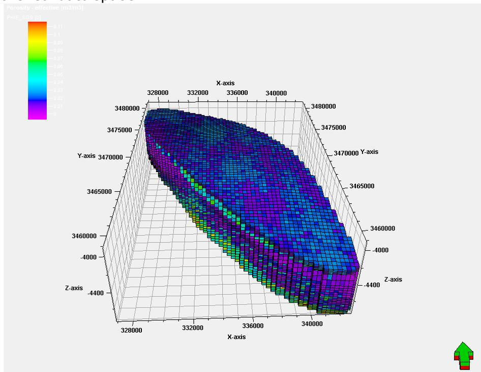
Figure 7. 3D modeling of porosity in Kupal oil field
