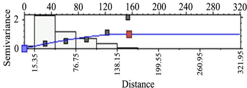
Figure 6. Variography model in the main-horizontal direction for porosity logs in zone 5
