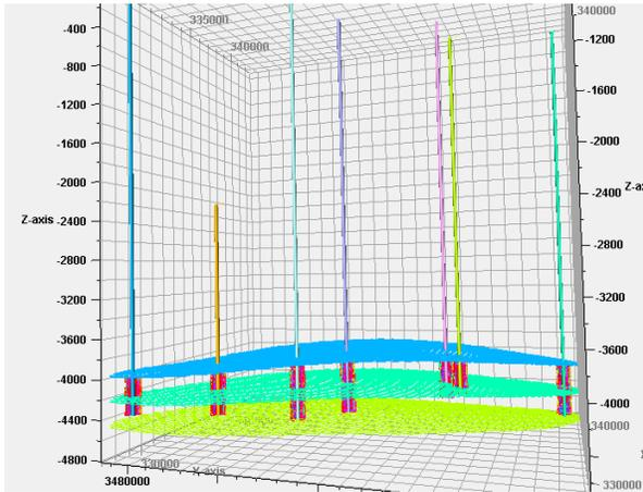
Figure 4. A view of created cellular network in Kupal oil field.
