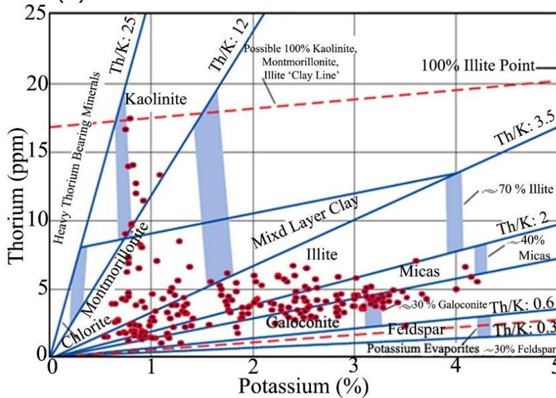
Figure 4. Identify the type of clay minerals for well No.54 in the Kupal oil field
