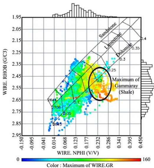
Figure 2. Cross plot of Neutron-Density-GR, Well No.54 in Kupal oil field
