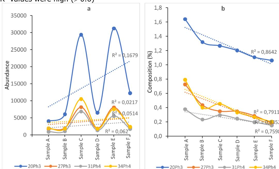
Figure 4. Plot of some C<sub>3</sub>-C<sub>4</sub> Phenanthrenes (20Ph3, 27Ph3, 31Ph4, and 34Ph4) against all the studied oil samples showing the level of correlation a. abundance b. composition
