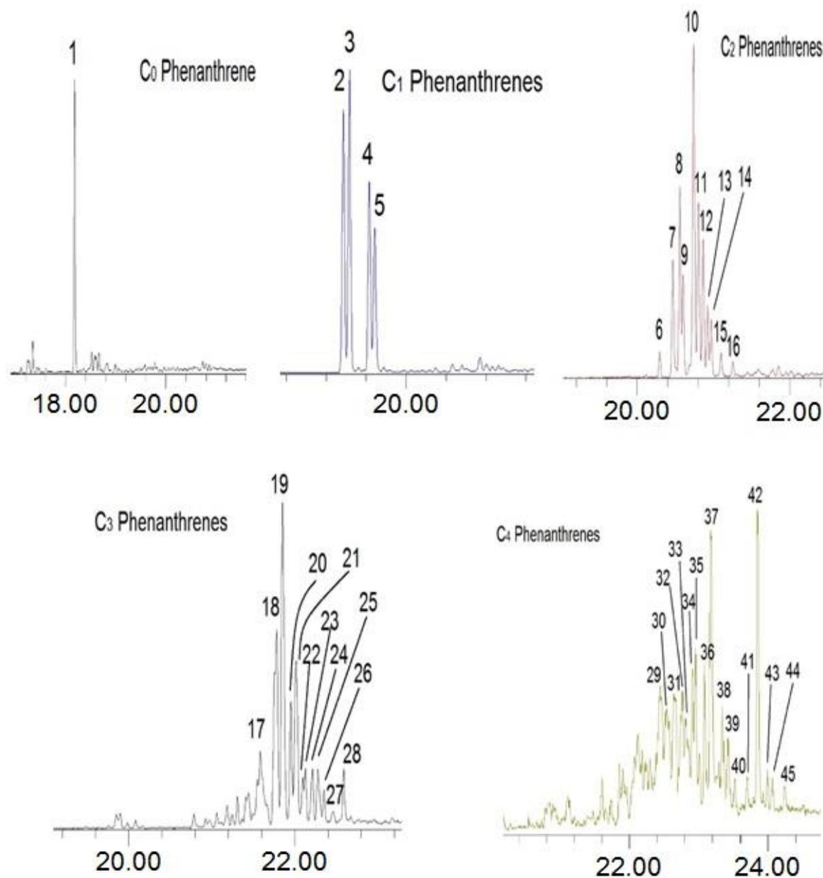
Figure 2. Representative GC-MS fragmentogram of  $C_0$ - $C_4$  phenanthrenes at ions ( $m/z$ ) 178, 192, 206, 220 and 234 showing the selected peak distributions in crude oil (sample B)
