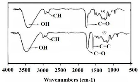
Figure 2. FTIR spectrum of (a) HB-(OH)8 and (b) H1 respectively
