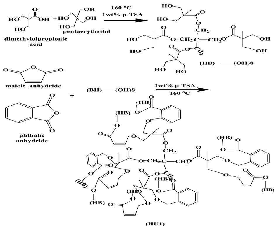
Figure 1. The schematic presentation of the synthesis of unsaturated hyperbranched nanoparticles
