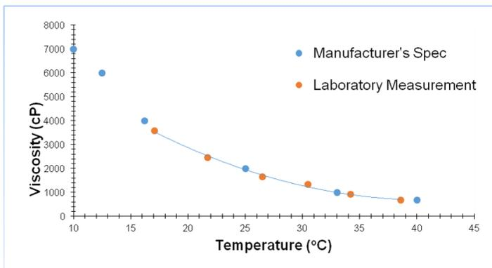
Figure 5. Comparison of oil viscosity measured and supplied by the manufacturer
