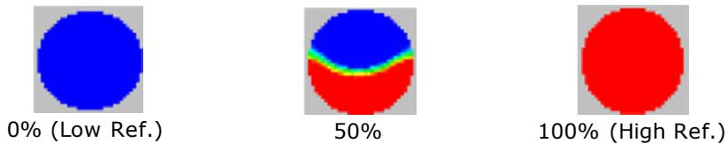
Figure 3. Tomographic images of liquid holdup
