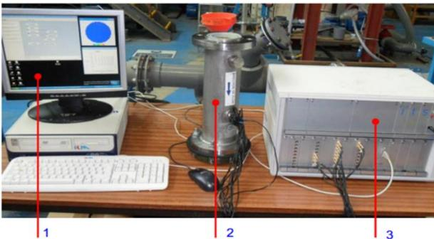
Figure 2. ECT System; (1)-Computer System, (2)-ECT Sensors embedded in the pipe and (3)-Data Acquisition System
