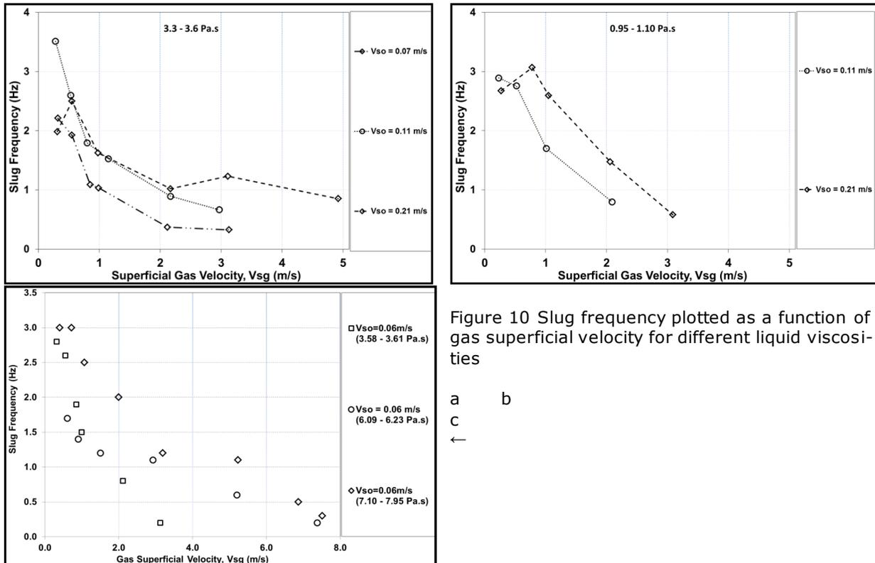
Figure 10 Slug frequency plotted as a function of gas superficial velocity for different liquid viscosities
