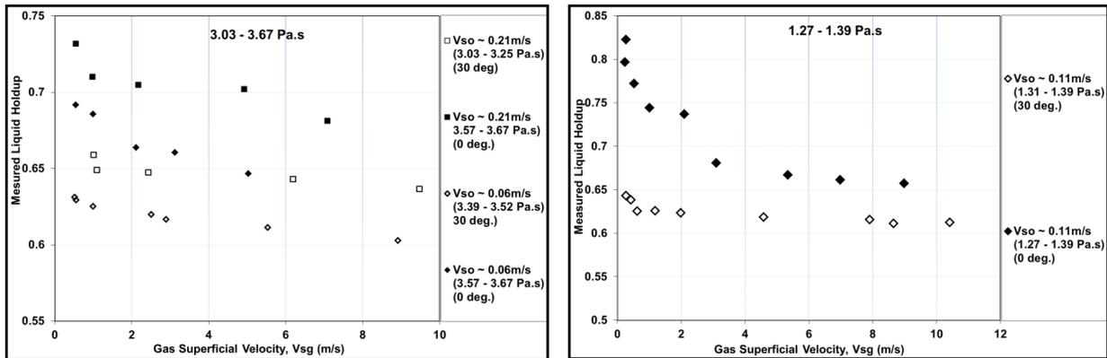
Figure 7. Effects of inclination on liquid holdup plotted as a function of superficial gas velocity for different oil viscosities (a/b)
