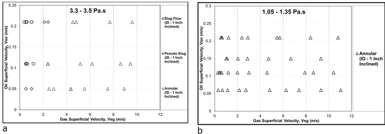
Figure 6. Flow pattern map for oil-gas two phase flows 1-inch inclined test section
