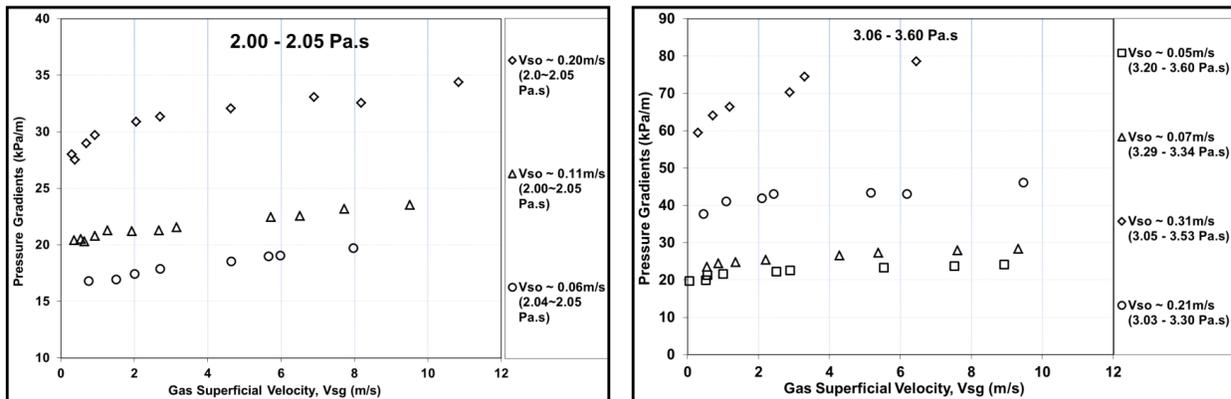
Figure 8. Pressure gradients as a function of superficial gas velocity (a/b)
