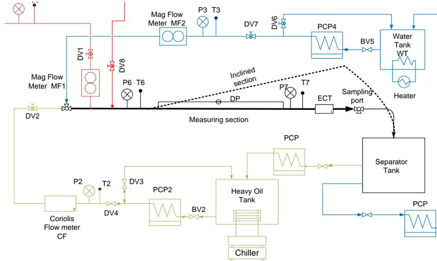
Figure 1. Schematics of the 1 inch test facility
