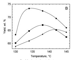
A-sulfated catalyst B-chlorinated catalyst Figure 2. Yield of C5-C6 isoalkanes depending on temperature:  $(\bullet)$  – composition No. 1,  $(\blacksquare)$  – composition No. 6
