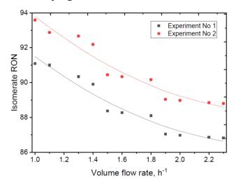
As the load on the raw material increases on the isomerization reactor unit, the contact time of the raw material with the catalyst decreases, and the octane number of the isomerizate obtained decreases. The forecast is based on models of the influence of feed loading on the octane number of the isomerized product to the isomerization with recycling of  $n-C_5-C_6$  and the low-branched hexanes presented in Fig. 3.
