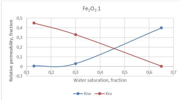
Fig. 11. Relative permeability curve at 1 wt. % Fe<sub>2</sub>O<sub>3</sub>
