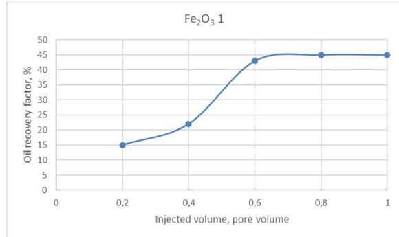
Fig. 12. Effect of 1 wt. % Fe<sub>2</sub>O<sub>3</sub> on oil recovery
