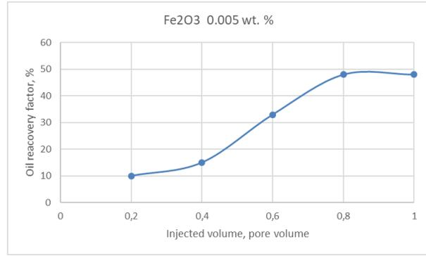
Fig. 5. Relative permeability curve at 0.005 wt %  $Fe_2O_3$  Fig. 6. Effect of 0.005 wt. %  $Fe_2O_3$  on oil recovery
