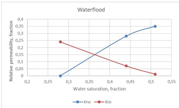
Fig. 3. Relative permeability curve for conventional water flooding
