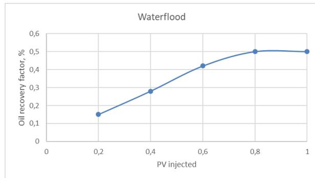
Fig. 4: Effect of conventional water flooding on oil recovery
