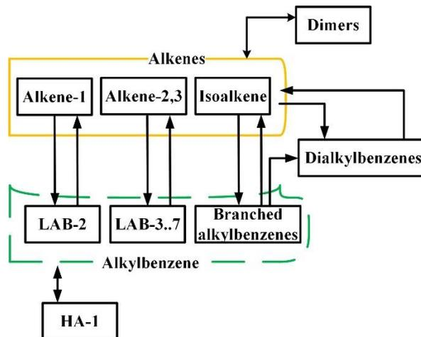
Figure 2. Reaction network of the alkylation process
