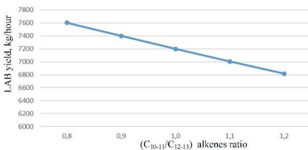
Figure 3. Yield of LAB depending on the ( $C_{10-11}/C_{12-13}$ ) alkenes ratio
